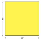
One side of the cube is made of a 4'x4' panel of Compbond aluminum composite panel. This size offers the option of activating the top. There are a total of (4) 16 sq ft surfaces for activation.
